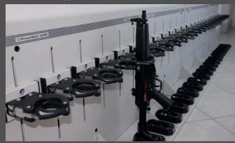
ALL THE WEAPONS ARE IDENTIFIED BY RFID TAG AND THE SYSTEM KEEPS TRACK OF THE WEAPON USAGE DOWN TO A USER AND ACCESS TIME LEVEL.
